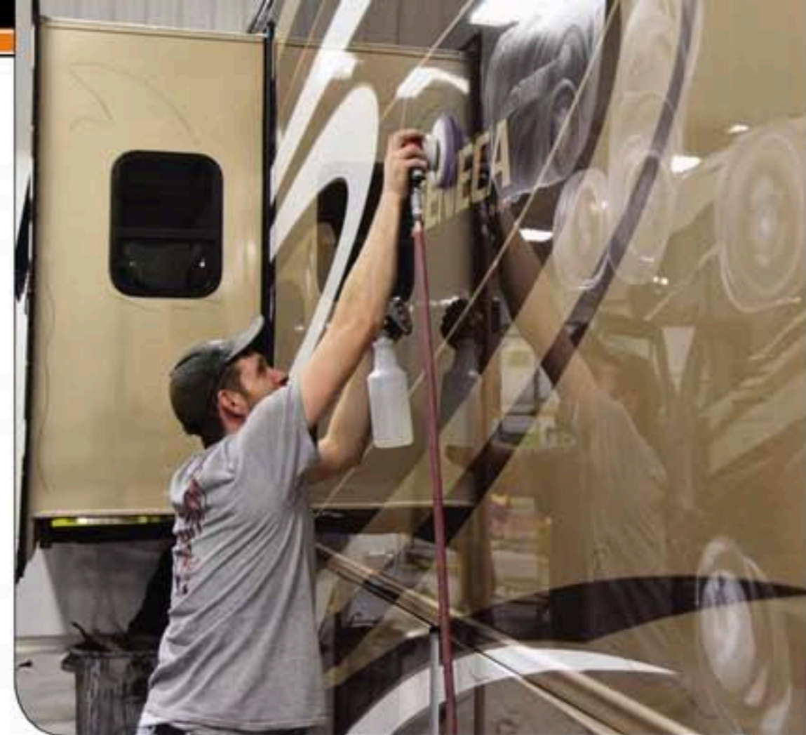
Precision Painting's Buffer Supervisor Allen Longacre sands an RV. It's the first stage in buffing after being clear coated.
